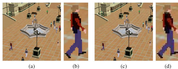
Fig. 4. Compression artifacts in synthetic video. (a) Uncompressed image. (b) Enlarged region of the rectangular box in (a). (c) JPEG-compressed image. (d) Enlarged region of the rectangular box in (c).
