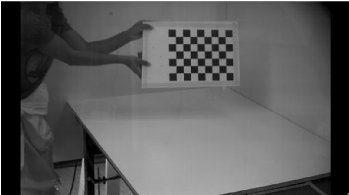
Figure 2.6: Still shot from a moving checkerboard calibration video. The checkerboard is moved around in the view of both cameras and the calibration program identifies the individual squares on the checkerboard. The image has been lightened to enhance contrast.
