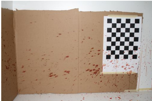
(a) Porcine bloodstain pattern photograph taken in a position in front of Camera A.
