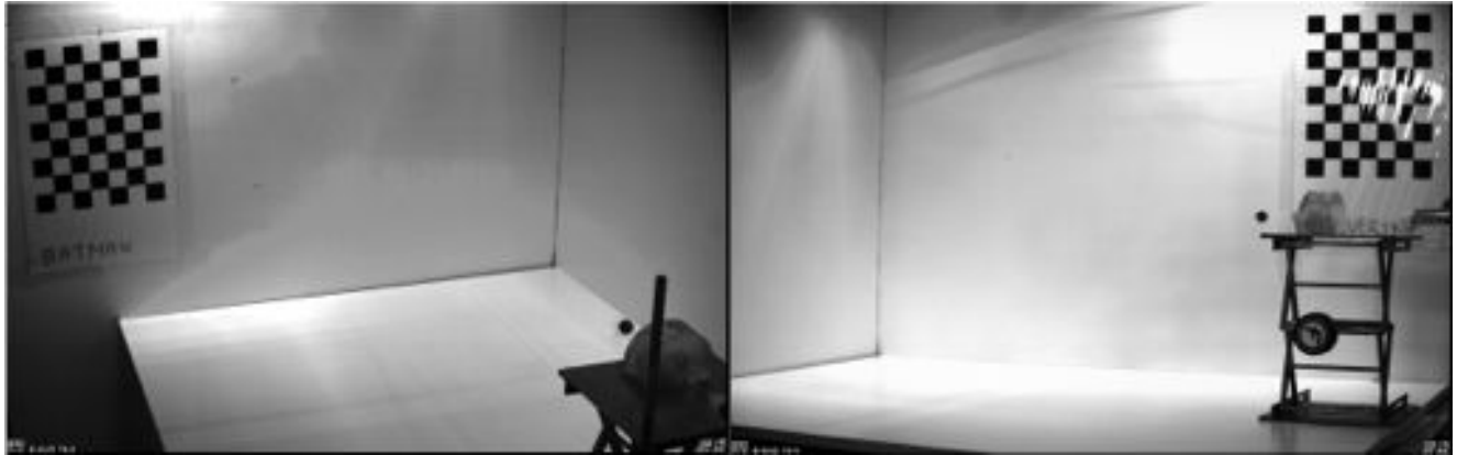
Figure 2.7: Still frame (as captured by both cameras) to illustrate the placement of the mounted checkerboards. Each camera captures only one checkerboard. In both views of the mock crime scene, the riot ball can be seen emerging from the ballistics gel. The figure on the left is a still shot from Camera B and the figure on the right is still shot from Camera A.
